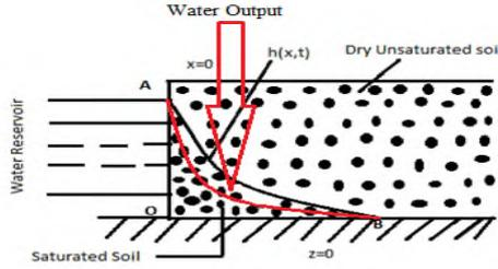
**Figure 4: Schematic figure of ground water infiltration when water output from the porous stratum by Sink or Pumping**
